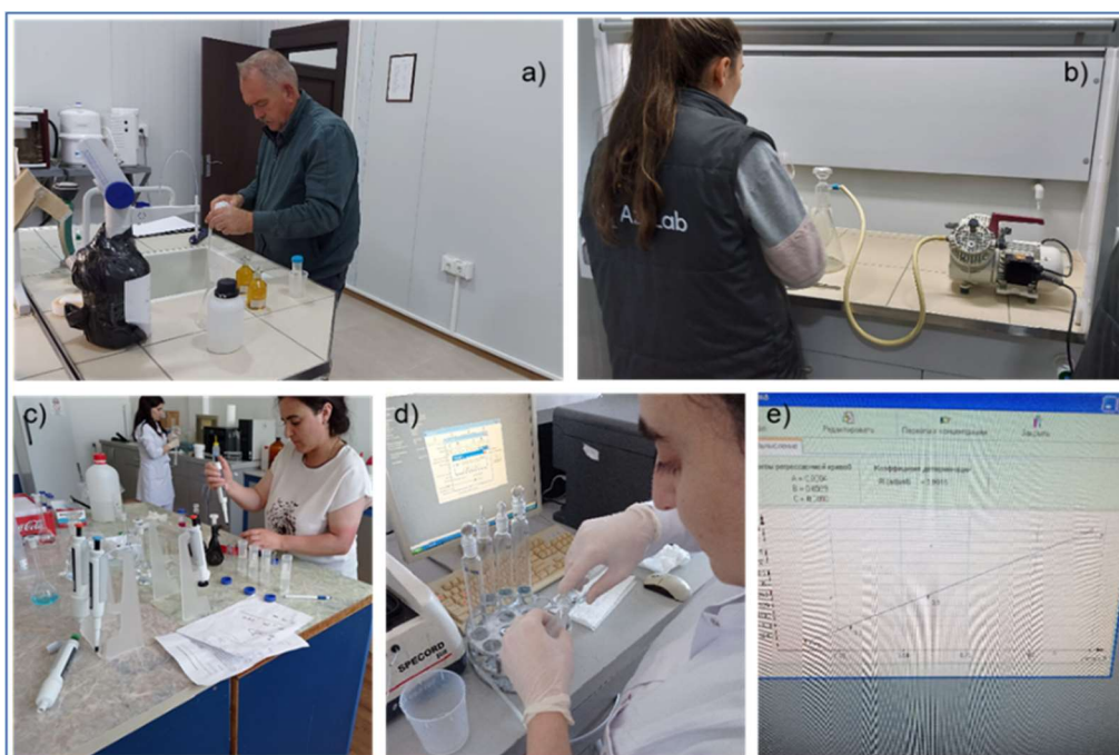
Figure 2: Determination of dissolved oxygen content by thiosulfate titration (a), filtration of samples through glass fiber filters for chlorophyll a determination (b), preparation of ammonia standards (c), spectrophotometric determination (d) and observed calibration line (e).
